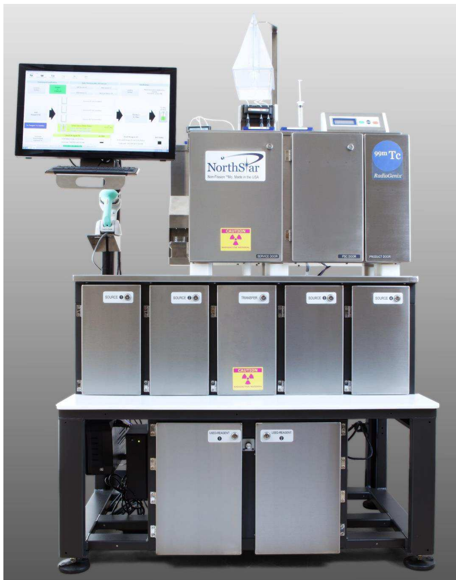
Figure 4. RadoGenix separator developed by NorthStar for separating ^{99m}\text{Tc} from a solution of ^{99}\text{Mo} . The unit is fully automated, operates at room temperature, does not require a fume hood and has a separation efficiency greater than 90 %. The required reagents are held in the clamshell structure at the top; the ABEC separation column is in middle unit on the top shelf and the ^{99m}\text{Tc} product is delivered to the module on the right; up to four ^{99}\text{Mo} sources can be loaded on the middle shelf; reagent waste is stored on the bottom shelf. The unit is presently undergoing assessment for US FDA approval. (Photo courtesy of NorthStar Medical Radioisotopes).
