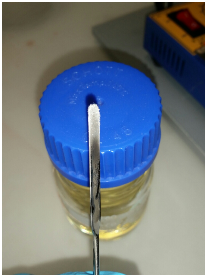
Figure S6. Photograph of a spatula upon which anthracene was deposited in our coating apparatus. The crystalline structure of the deposit is clearly visible. The conditions used for this experiment were used for the experiment labelled Path SS in Figure 2.
