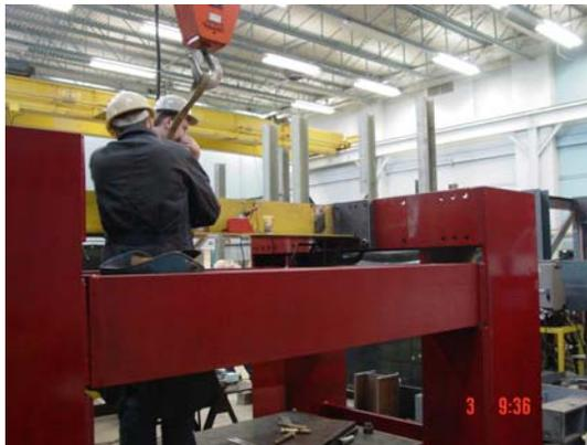
Figure 4. Preparations for testing final single frames in the grillage support frame.
