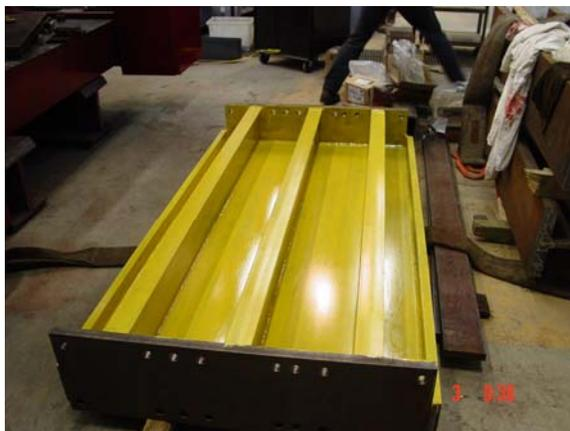
Figure 5. Small grillage ready for application of strain gauges.
