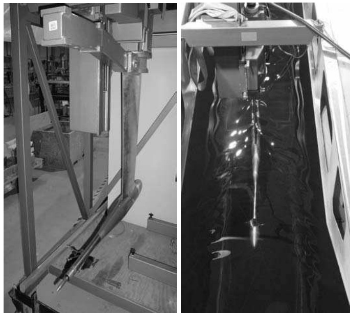
Figure 5. Kempf & Remmers dynamometer: in test frame (left) and in the tow tank (right).
