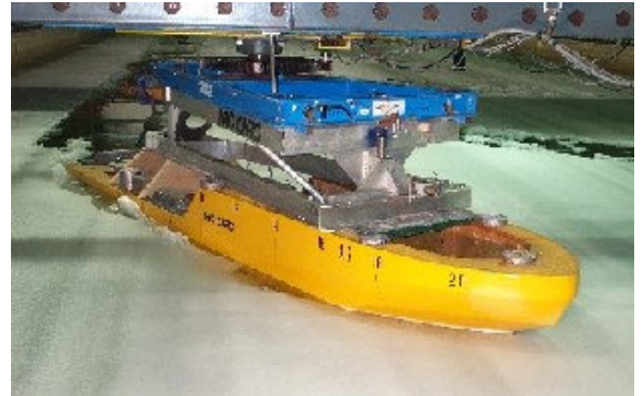
Figure 2: Terry Fox model attached to the PMM.
