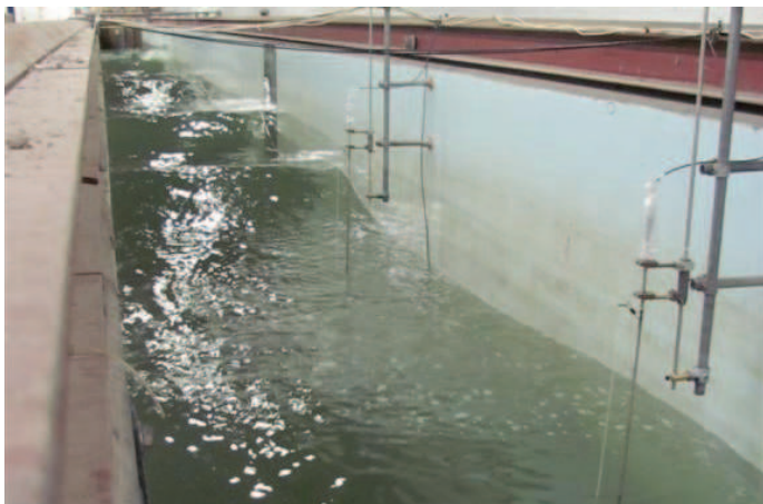
FIGURE 4. 2D TESTING IN A 97M X 2M WAVE FLUME.
