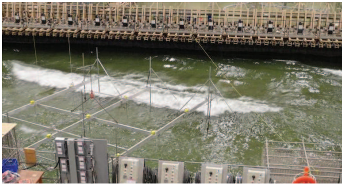
FIGURE 3. 3D TESTING IN A 36M X 30M MULTIDIRECTIONAL WAVE BASIN
