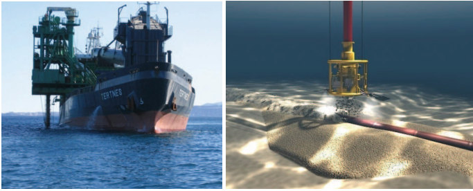
FIGURE 2. FALL PIPE VESSEL AND ILLUSTRATION OF ROCK PLACEMENT
