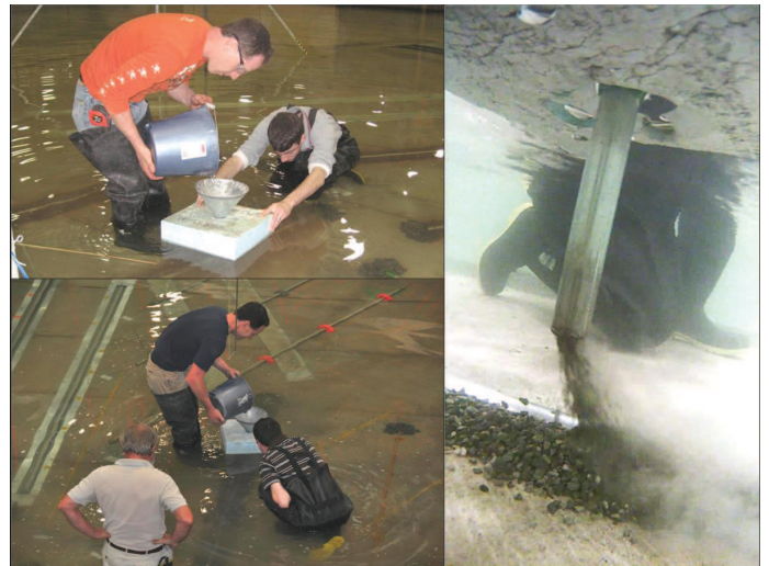
FIGURE 6. SIMULATION OF ROCK BERM CONSTRUCTION BY FALL PIPE
