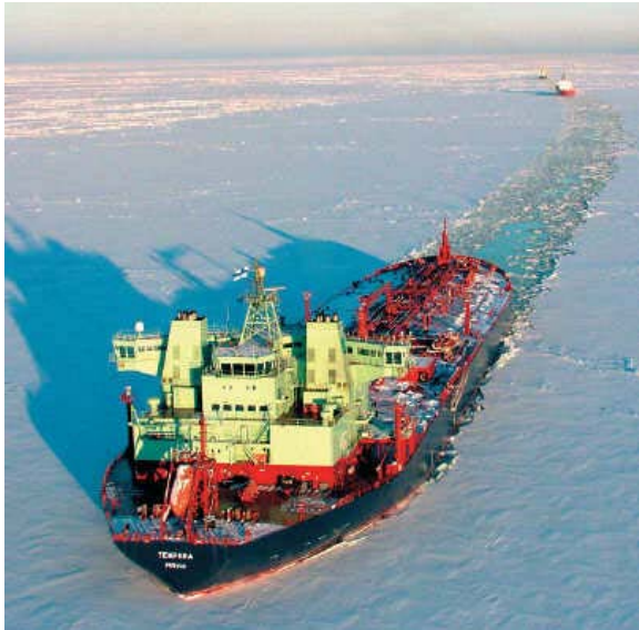
Fig. 15. A 106,000-dwt Masa-Yards-developed DAT crude carriers built by Sumitomo Heavy Industries in 2003.
