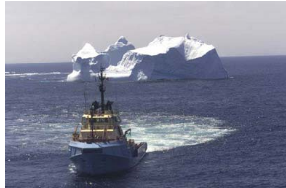
Fig. 21. Towing a medium sized iceberg off Newfoundland
