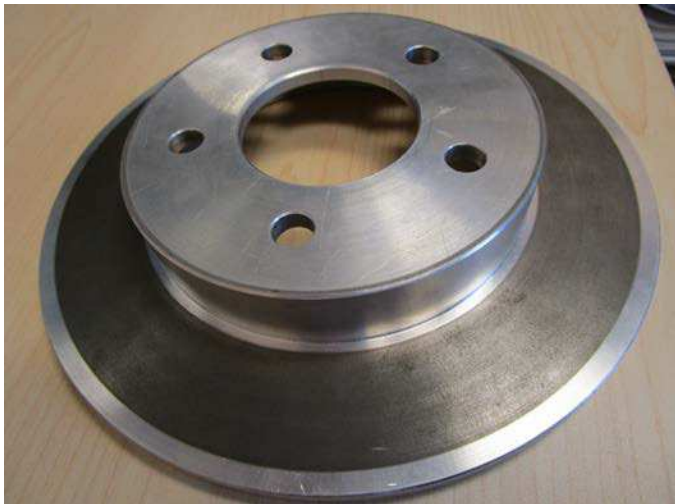
Figure 6: Picture of the prototype disk (coating is darker than the Al disk)
