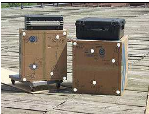
Figure 18: Demonstration under sunlight illumination and analysis of worst case scenarios of on-orbits light conditions. This was accomplished by comparing the tracking while removing the optical interference filter inside the laser scanner head.
