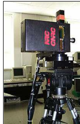
Figure 3: Prototype of the 3-D Laser Scanner System.
