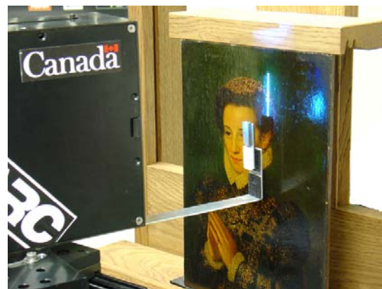
Figure 2: Prototype of the laser scanner system.
