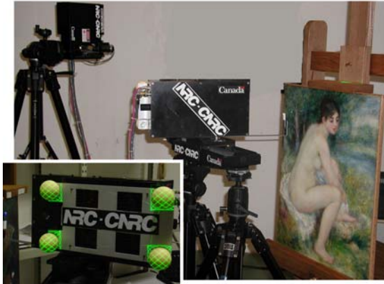
Figure 3: The 6 DOF positioning of the High-Resolution Color System (foreground) is monitored in real-time by the large volume system (background). Bottom-left Lissajous tracking pattern on the sphere.
