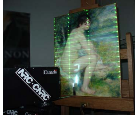
Figure 4: The tracking system monitors the position of the painting and automatically generates a grid pattern. Each grid accurately indicates the sections to be scanned to minimize the overlay. The tracking system also records the overall shape of the painting to a resolution of 200 \mu\text{m} .
