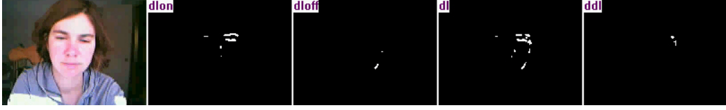
Figure 4: Detecting changes in the face of the user, while she is winking with her left (right in the figure) eye: the first order change image dI , which is made by combining positive dI_{on} and negative dI_{off} change images, is decomposed into a long lasting change (not shown) dI_{long} and the most recent change ddI (shown at right). dI_{long} image can then be used to remove from dI_{on} and dI_{off} images those pixels which have changed due to the head motion.
