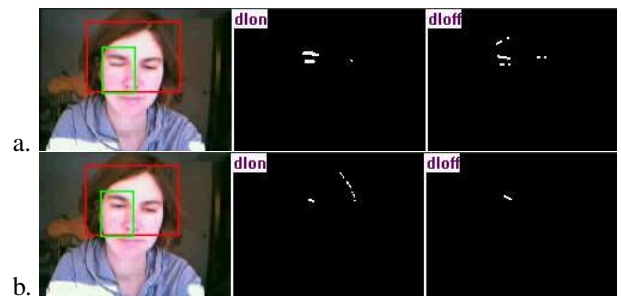
Figure 7: Analyzing different regions of the change images can be used to discriminate a wink from head motion: in (a) a person winks with her left (right in the image) eye, in (b) she slightly moves her head..
