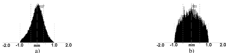
Figure 1 - Example of a histogram of residual errors after alignment of 2 images: a) best possible calibration, b) poorer calibration.
