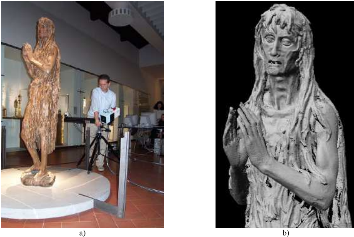
Figure 2 - 3D scanning: a) relocation of the 3D scanning system around the statue, b) 3D model
