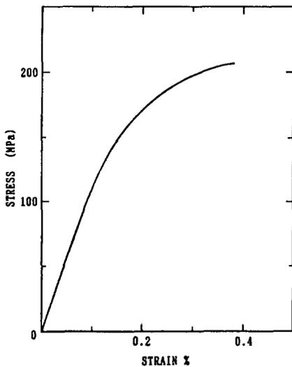
Fig. 5 Typical tensile stress-strain curve of the Al<sub>7</sub>Ti<sub>25</sub>Mn<sub>8</sub> alloy, 70% hot-pressed and 1273K/2h annealed
