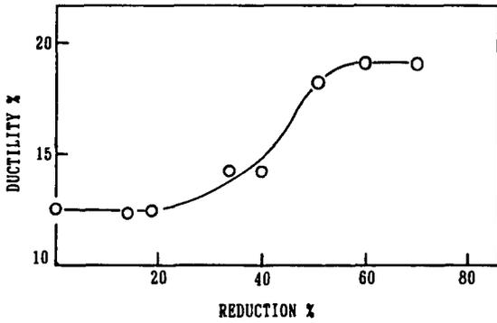
Fig. 3 Room temperature compressive ductility of hot-pressed and annealed Al<sub>7</sub>Ti<sub>25</sub>Mn<sub>8</sub> alloy as a function of reduction
