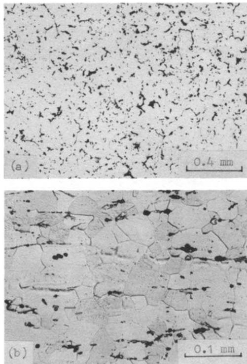
**Fig. 2** Micrographs of induction-melted  $Al_{67}Ti_{25}Mn_8$  alloy (a) as-cast and homogenized (b) 70% hot-pressed and 1273K/2h annealed
