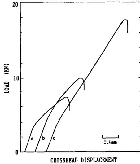
Fig. 4 Typical load-deformation curves of the Al<sub>7</sub>Ti<sub>25</sub>Mn<sub>8</sub> alloy compression tested at room temperature
