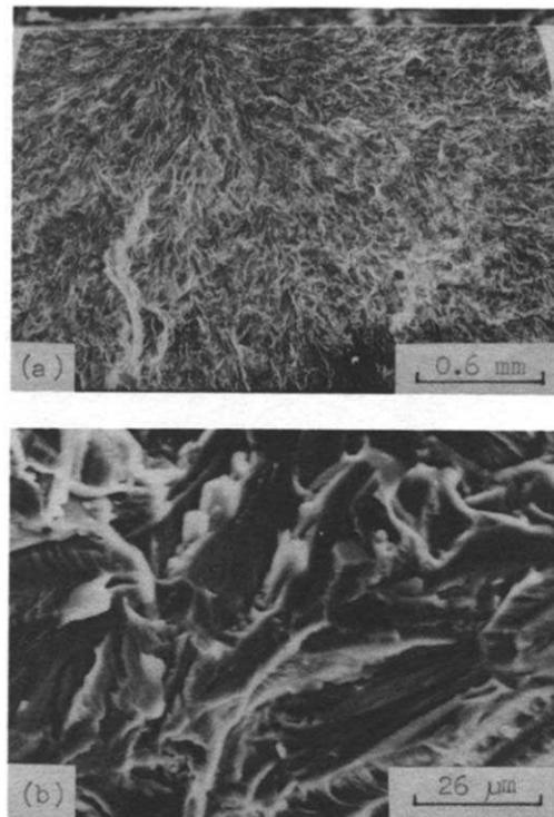
Fig. 6 SEM fractographs of tensile tested specimen of Al<sub>7</sub>Ti<sub>25</sub>Mn<sub>8</sub> alloy
