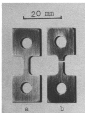
**Fig. 1** Tensile specimens of  $Al_{67}Ti_{25}Mn_8$  alloy (a) before and (b) after test
