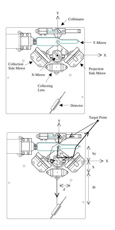
Figure 1. Top views of the LCS baseplate and its various components. The projection and collection paths are shown in solid and dotted lines, respectively. The parameters studied during the sensitivity analysis are:  $\alpha c$ : collection side mirror angle;  $\alpha p$ : projection side mirror angle; f0: distance between the collecting lens and the detector; d: half-baseline; S: distance between the X-mirror pivot and the collecting lens; hy: distance between the X-and Y-mirror pivots.
