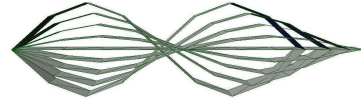
Figure 2: Most isometric morph of a simple polygon. The start polygon is a 3D polygon obtained by discretizing the curve y = \sin(x) and by adding thickness to the curve along the z -direction. The end polygon is similarly obtained from y = -\sin(x) .
