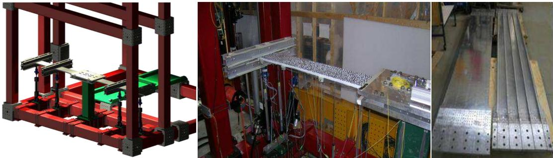
*Figure 2: Simple beam and Z stringer stiffened aircraft skin bending and torsion platform for evaluating load monitoring technologies.*
