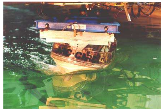
Figure 7, Escort tug model tested on Planar Motion Mechanism
