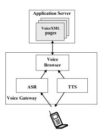
Figure 1. VoiceXML architecture model
