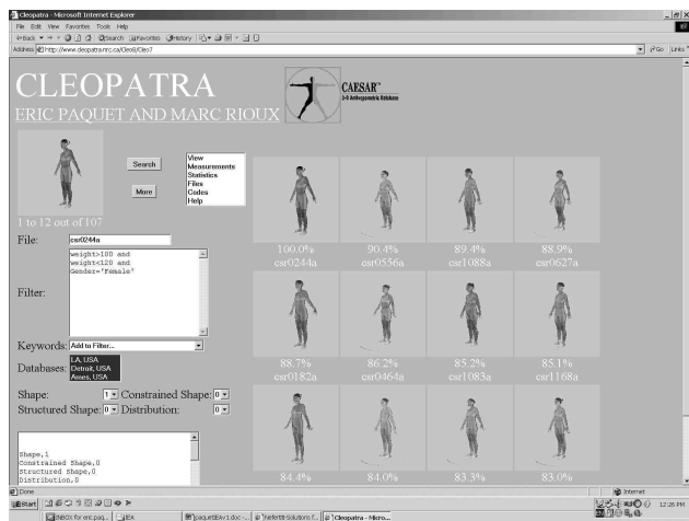
Figure 1. Outcome of a query for a thin woman from the CAESAR™ database with our three-dimensional shape content-based approach. Constraints have been applied on the weight and the gender.
