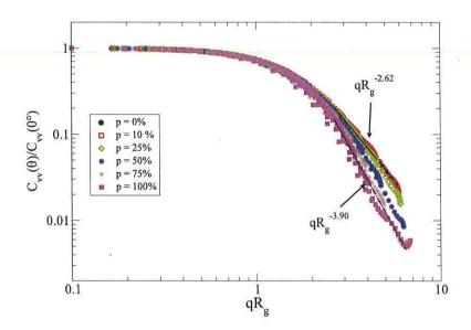
Fig. 4 Impact of coating on the normalized vertical-vertical differential scattering cross section (structure factor) for the largest aggregate ( $N_p = 96$ ) considered. Results at all the seven wavelengths investigated are included.
