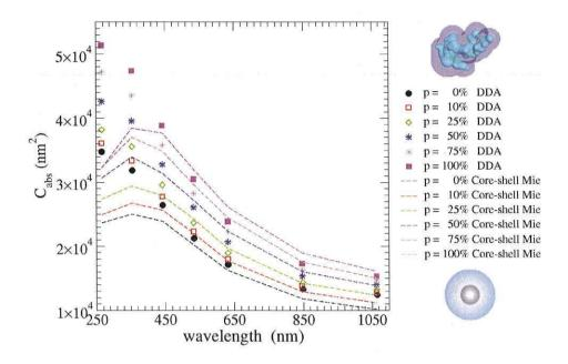
Fig. 10 Comparison of the absorption cross sections predicted by DDA and core-shell Mie at coating levels of 0 from to 100% for  $N_p = 96$ .
