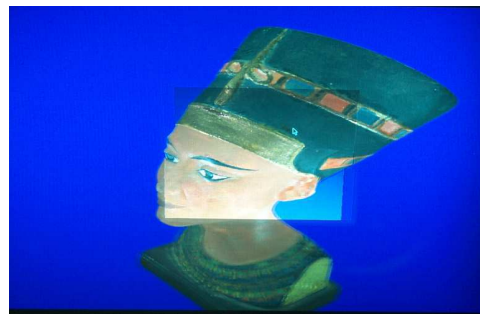
Figure 6. Stereoscopic dual-resolution display with adaptive boundaries (photograph of the screen with superimposed left and right views).
