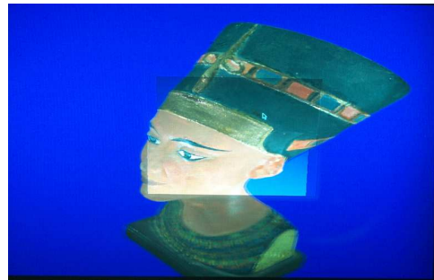
Figure 6. Stereoscopic dual-resolution display with adaptive boundaries (photograph of the screen with superimposed left and right views).
