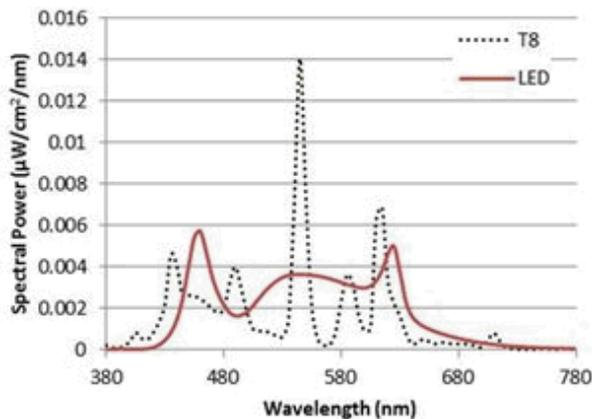
Figure 2. Spectral output of the existing T8 fluorescent lamps and LED retrofit luminaires.
