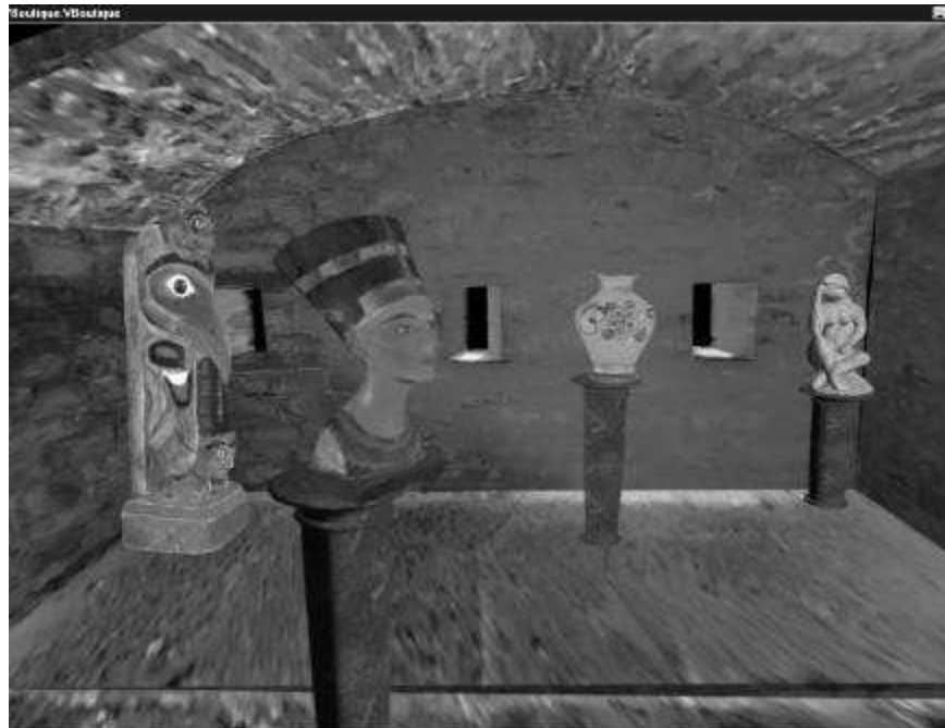
Figure 9. Virtualisation of a medieval room for the Virtual Boutique by photogrammetry. Only two pictures were used in the modelling process.
