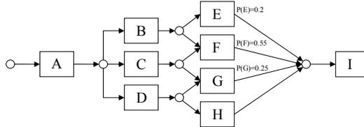
**Fig. 2.** Example Petri net showing the belief state for an event  $x$  that is believed to follow either task  $B$  or  $C$  and precede task  $I$ .
