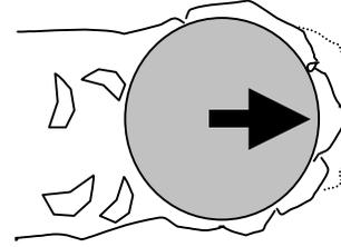
**Figure 3: Stress concentrators and subsequent cusp formation**
