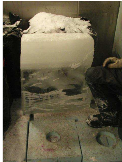
Figure 2: White ice (from flooding operations) on top of clear ice in a large block, collected from the Rideau Canal skateway, in Ottawa.
