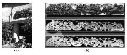
**Figure 4.** The Large Field of View camera is shown (a) mounted on a telescoping tripod to scan the sculpture *Mythic Messengers* at the Canadian Museum of Civilization. The sculpture, shown in (b, top), is mounted 4 m above ground on an exterior wall and measures 9 m long x 1. 2 m high. Over 100 scans were recorded as shown in the colour-coded image (b, middle) and merged into a 3D model (b, bottom). The data was then used to fabricate an accurate scale replica.
