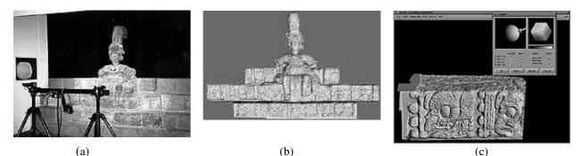
**Figure 3.** The Biris camera mounted on a linear translation stage (a) was used to scan the 3.4 m wide x 2.3 m high Hieroglyphic Stairway at the Peabody Museum in Boston to produce a 3D digital model (b). The software also enables the data to be used for research applications. Similar to the use of raking light to examine details on works of art, researchers can interactively move the light source to any angle and zoom in to examine features such details on the steps (c).
