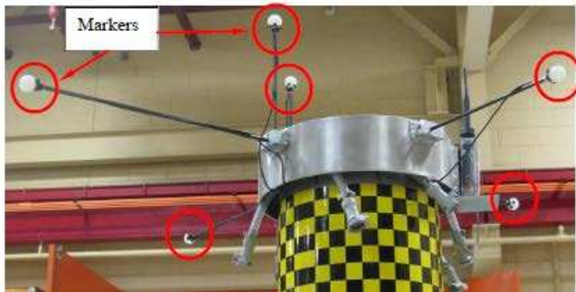
Fig. 8- The six Qualisys™ markers used in the model
