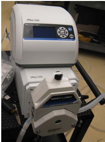
Fig. 5 - Masterflex™ I/P Precision Process Pump
