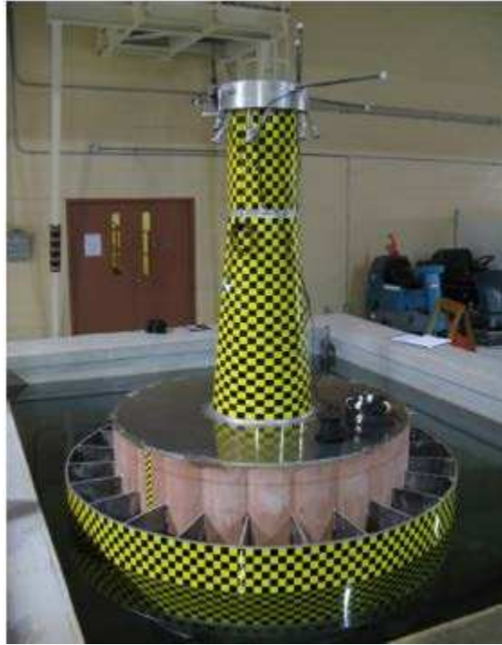
Fig. 6- A view of the model at the trim tank at NRC
