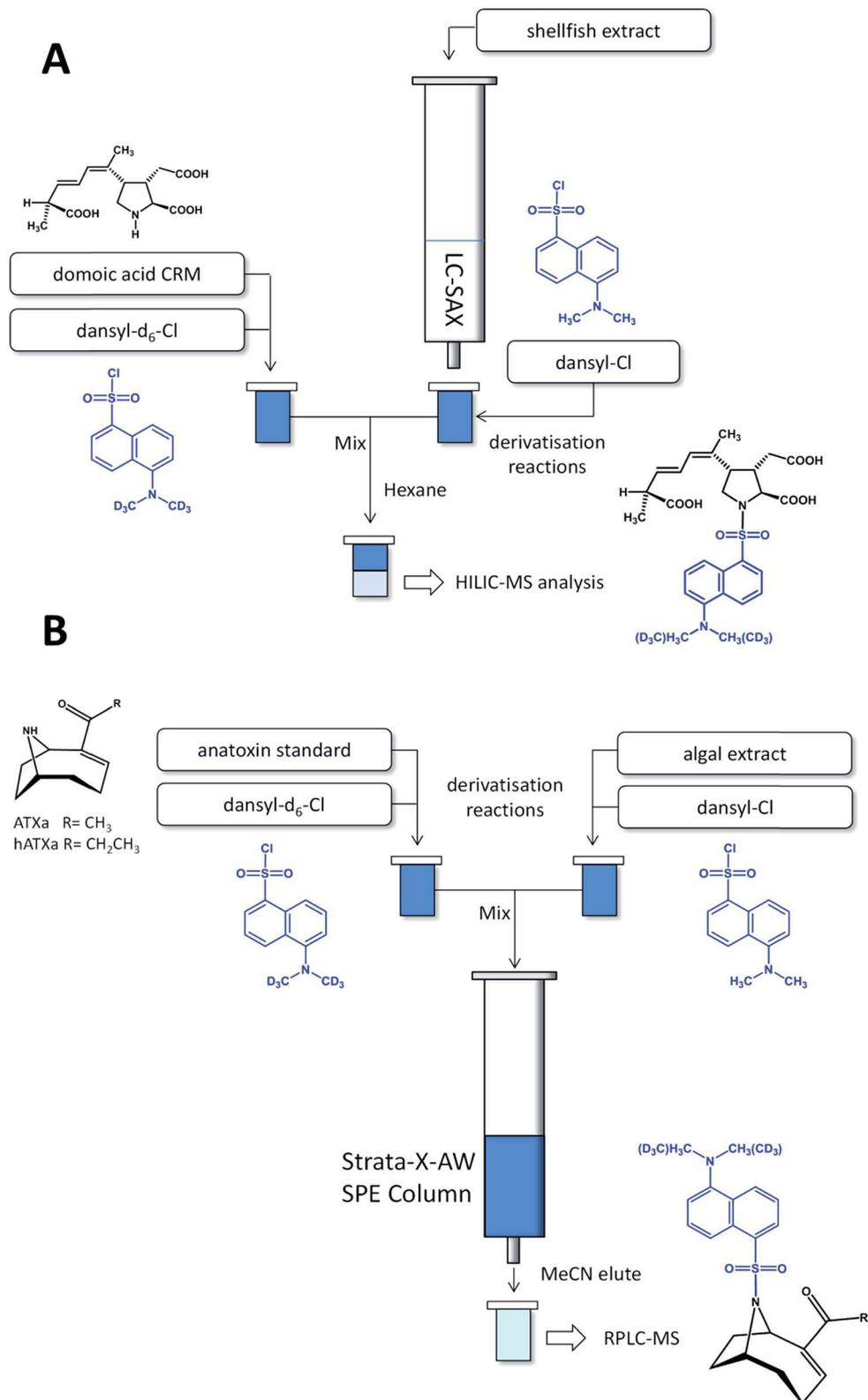
**Fig. 1** Schematic representation of sample clean-up and differential derivatisation procedures used for (A) DA in mussel tissue extracts and (B) ATX-a and hATXa in algal samples. Dark blue colour symbolises excess dansyl chloride derivatising agent that was removed prior to analysis.
