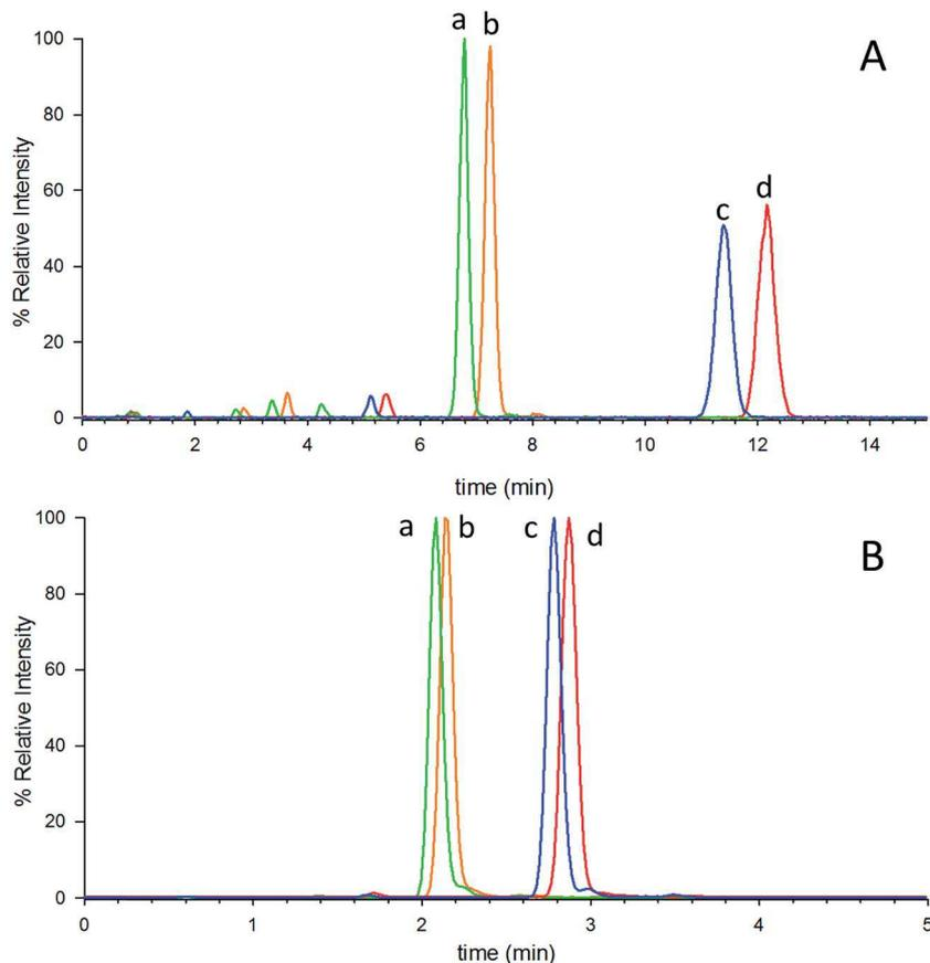
**Fig. 3** LC-MS/MS analysis of differentially dansylated anatoxins in algal extract showing separation of DNS- $d_6$ -ATXa (a) from DNS-ATXa (b) and DNS- $d_6$ -hATXa (c) from DNS-hATXa (d) using RPLC with 50% acetonitrile mobile phase (A). Separation of differentially labelled derivatives is minimised using 70% acetonitrile (B).
