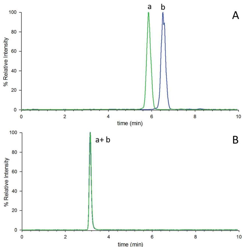
Fig. 2 LC-MS/MS analysis of differentially dansylated domoic acid in mussel tissue extract showing separation of DNS- $d_6$ -DA (a) from DNS-DA (b) by RPLC (A) and their co-elution by HILIC (B).
