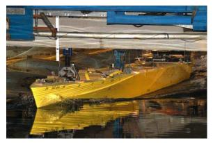
Figure 4: Bare Hull Resistance Test
