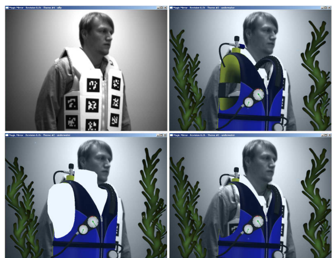
Figure 7: Usage of “dark matter” to provide correct occlusion relationship. Upper left: input camera image. Upper right: image after augmentation is naively added on top of image. Note the incorrect occlusion relationships such as the scuba tanks drawn in front of the body. Lower left: “dark matter” object drawn to approximate torso shape. Lower right: “dark matter” object not rendered to image but drawn to z-buffer allowing torso region to approximate correct occlusion by the body.
