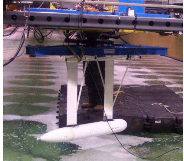
Fig. 2. The model installed on the PMM using the two vertical struts
