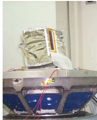
Figure 11. The Neptec Laser Camera Tracking System under vibration tests at the David Florida Laboratory (photo courtesy Neptec).
