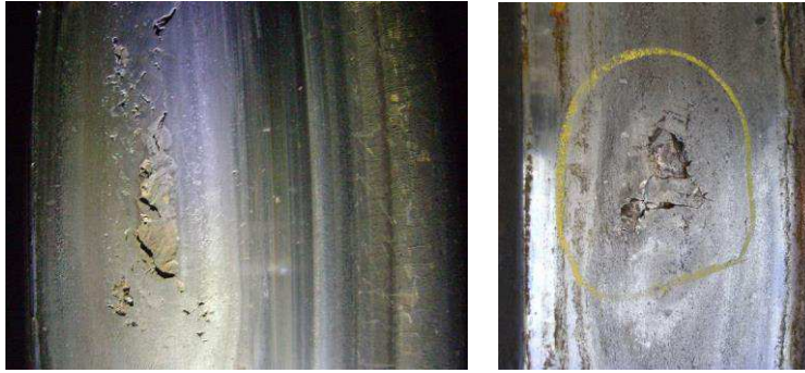
Figure 2: Examples of shelling on coal car wheels.
