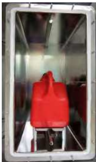
Figure 14: A test product with a cap on in a 50 L chamber vertically oriented
