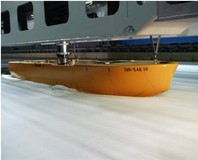
Fig. 1. Model 546 of the USCGC Healy in the ice tank at IOT.
