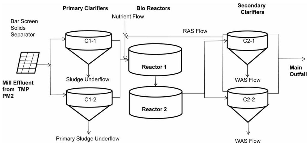
Figure 1 | A flow diagram of Port Hawkesbury Paper secondary treatment plant.
