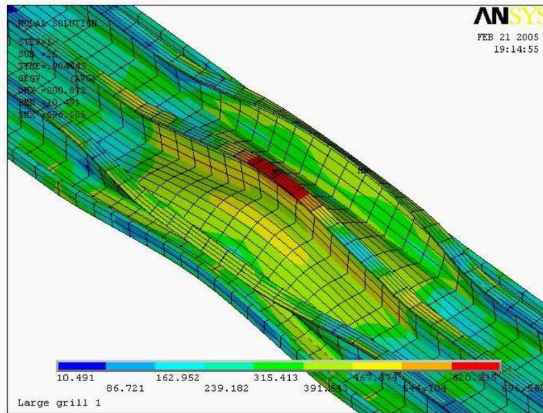
Figure 11. Large Grillage model with the load patch at a pressure of 18 MPa.
