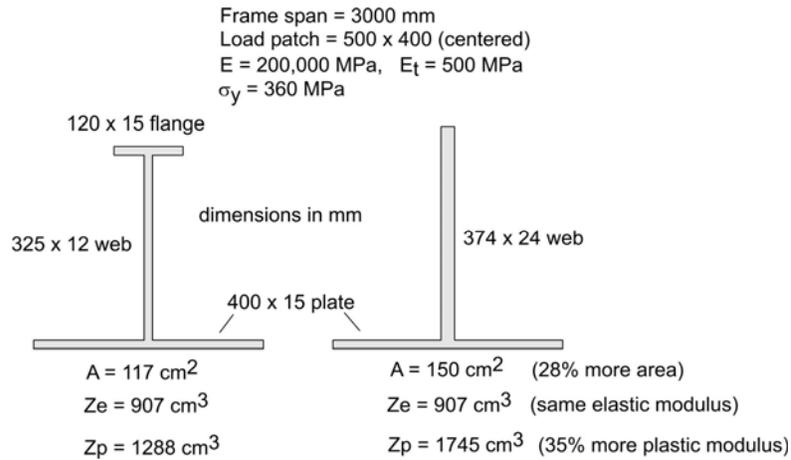
Figure 1. Two frames with equal elastic modulus.
