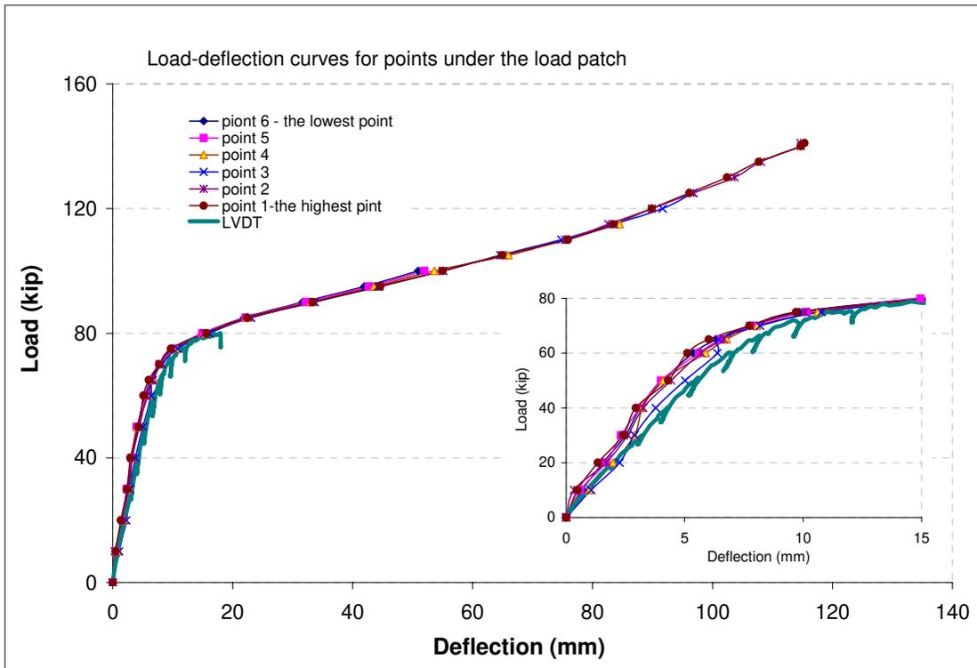
Figure 22. Measured load-deflection curves for end-loaded flat bar frame.
