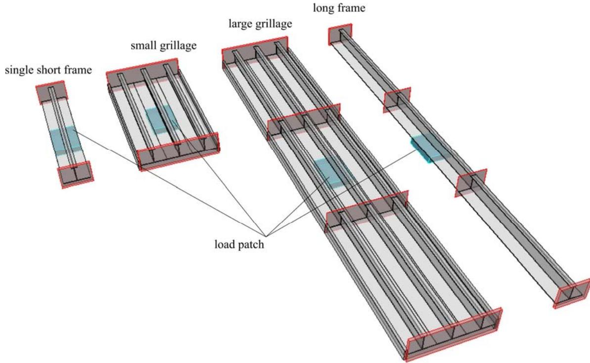
Figure 8. Four finite-element model frame arrangements showing load patch.
