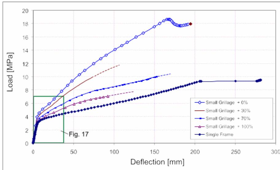
Figure 16. Load-deflection curves for the small grillage with varying load % on neighboring frames.
