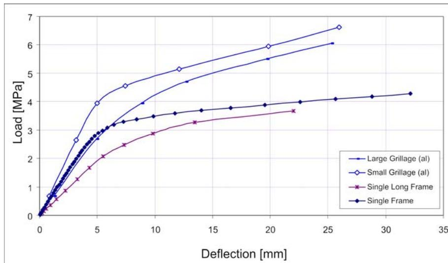
Figure 14. Initial portion of the load-deflection curves for the four configurations.
