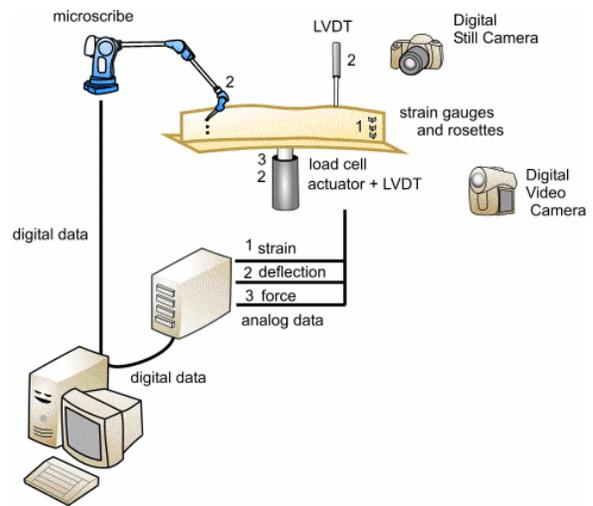
Figure 6. Data acquisition system for single frame tests.
