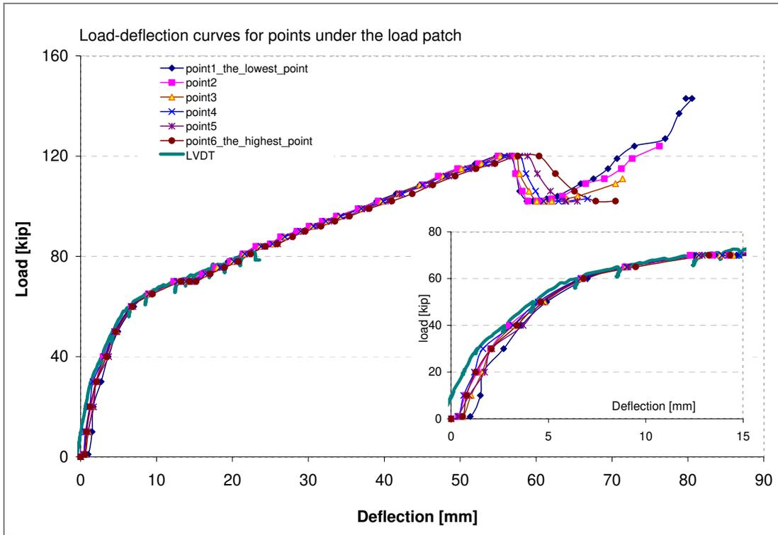
Figure 21. Measured load-deflection curves for end-loaded tee-75 frame.
