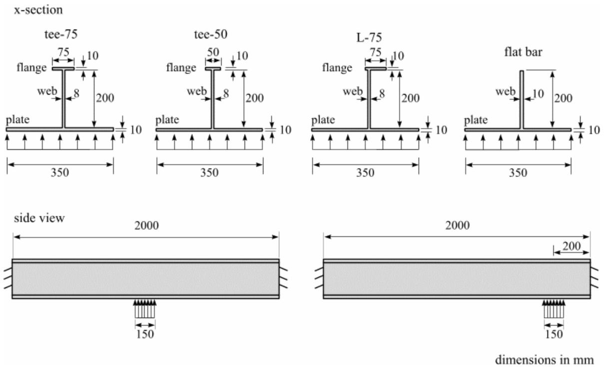
Figure 7. Basic Frame Dimensions for Single Frame Tests
