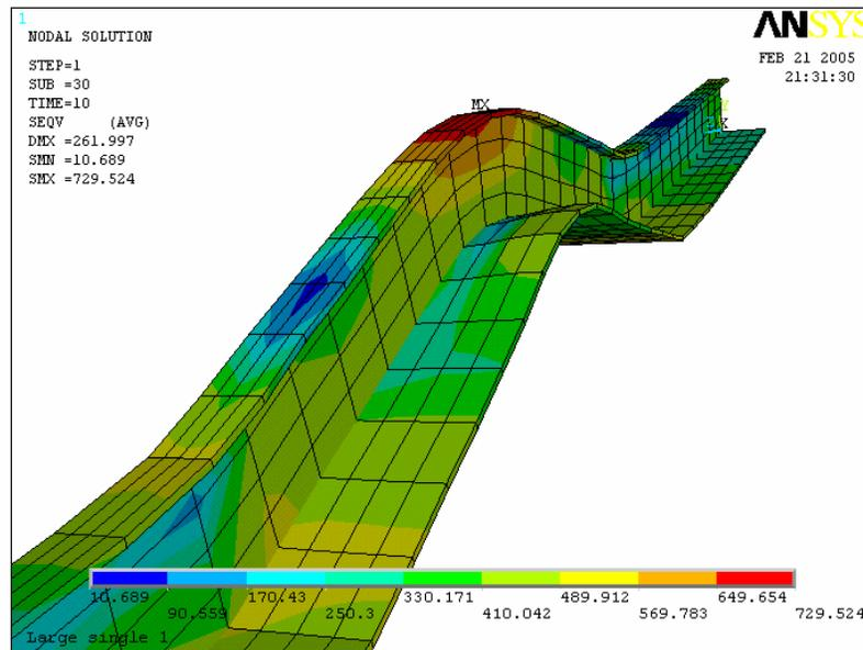
Figure 12. Long Frame model with the load patch at a pressure of 10 MPa.
