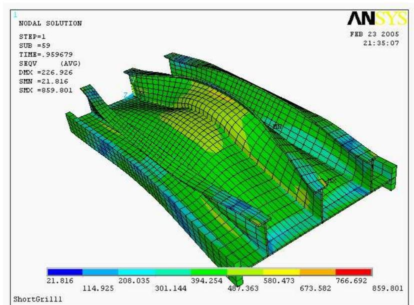
Figure 10. Small Grillage model with the load patch at a pressure of 19.2 MPa.
