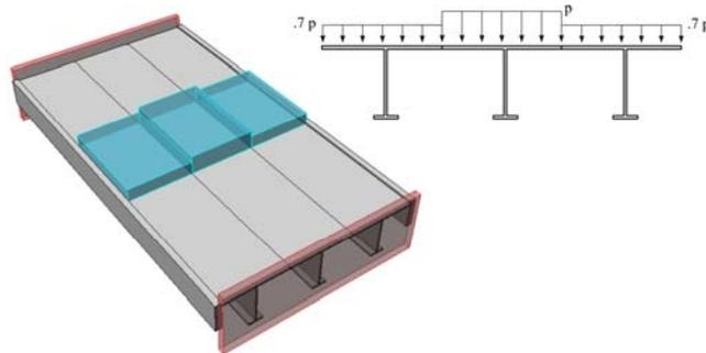
Figure 15. Load pattern on the small grillage with 70% load on neighboring frames.
