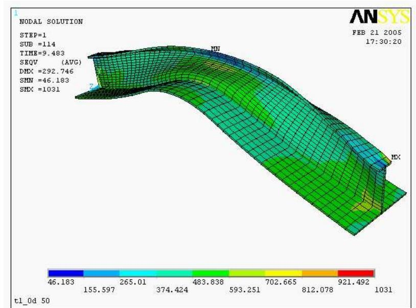
Figure 9. Single frame model with the load patch at a pressure of 9.483 MPa.
