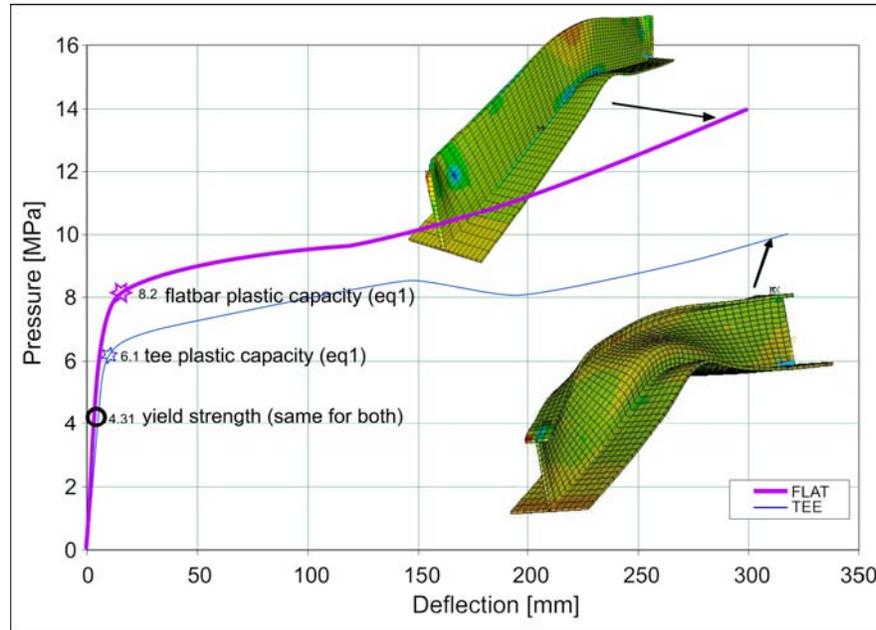
Figure 2. Comparison of load-deflection behaviour of two equal modulus frames.
