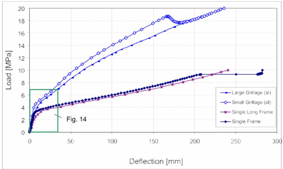
Figure 13. Comparison of the load-deflection curves for the four configurations.
