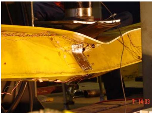
Figure 18. Tee-75 central load test.
