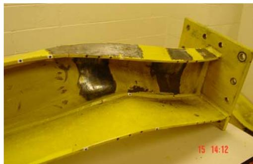
Figure 20 Tee-75 end load test.
