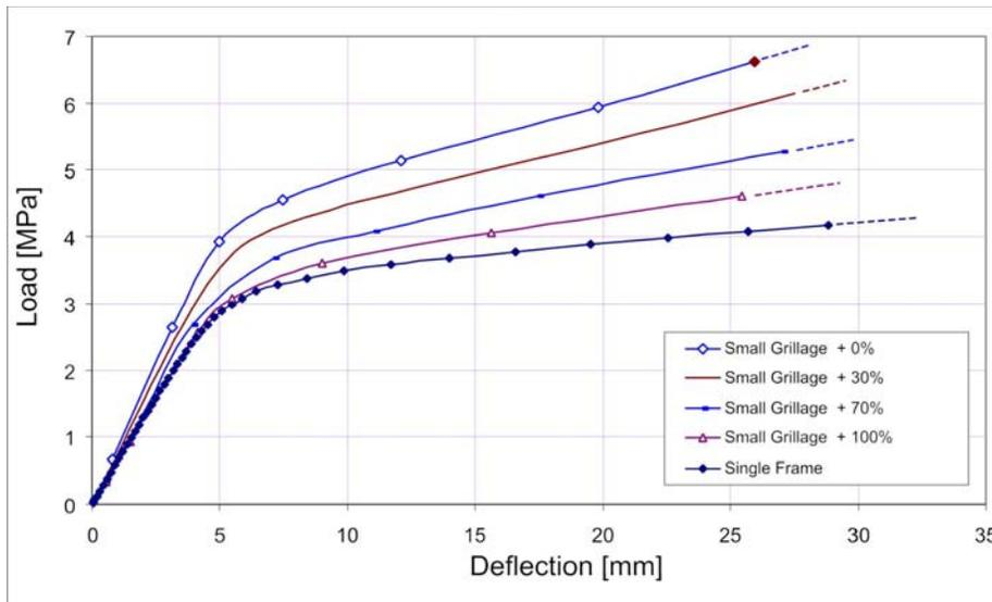
Figure 17. Initial portion of the load-deflection curves for Figure 16.
