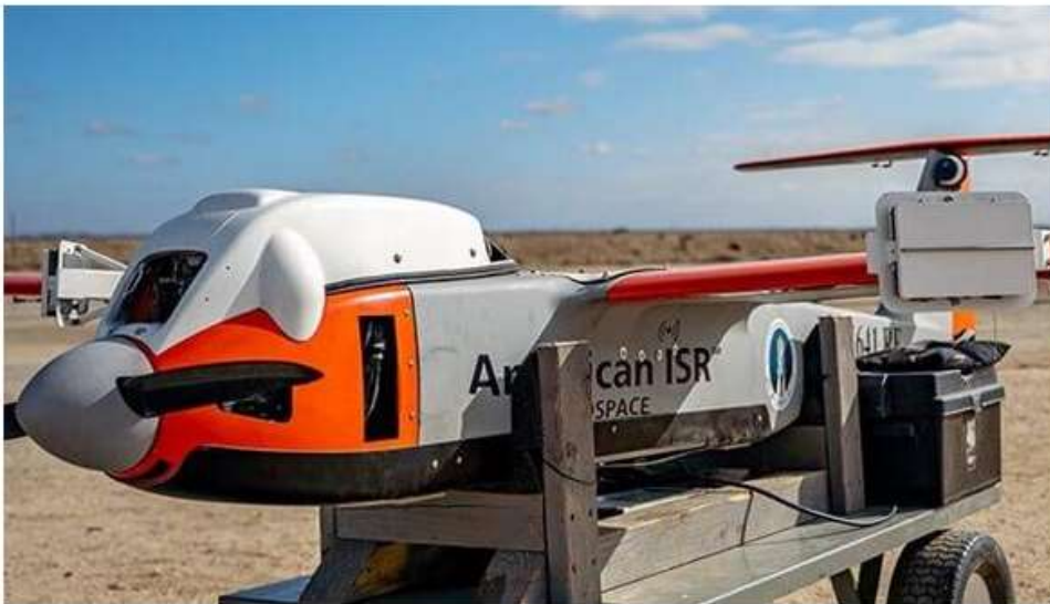
Figure 4 UAS platform (and Echodyne radar) used for NASA BVLOS aerial inspection demonstration [5].
