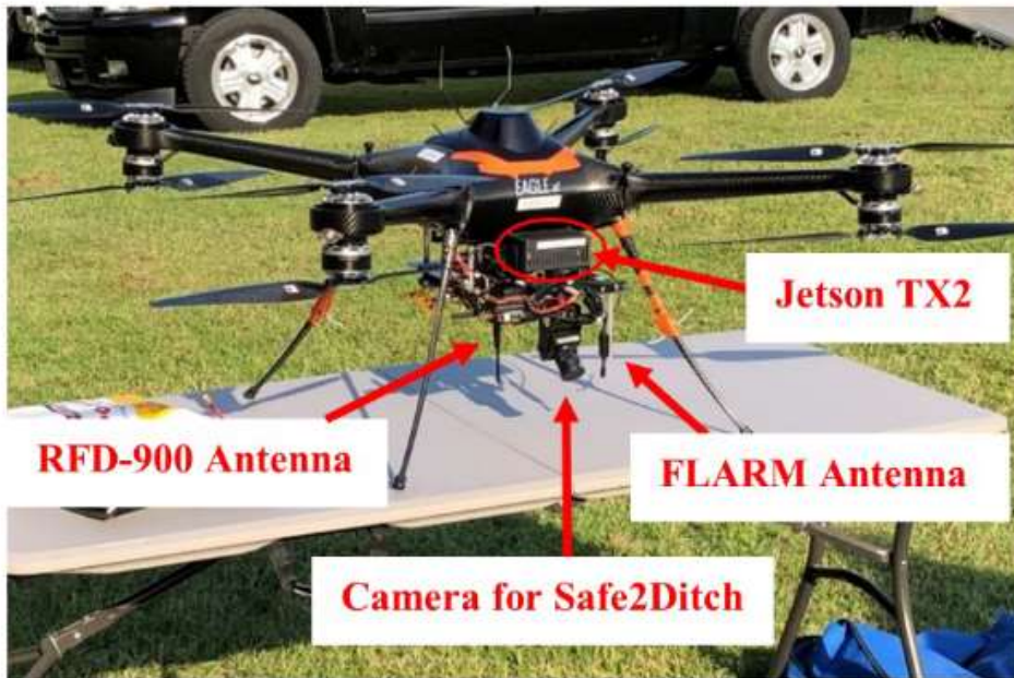
Figure 5 UAS platform used by NASA for DAA demonstration using FLARM [7]
