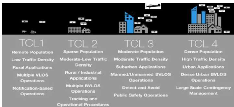
Figure 2: NASA UTM Technical Capability Level structure [3].
