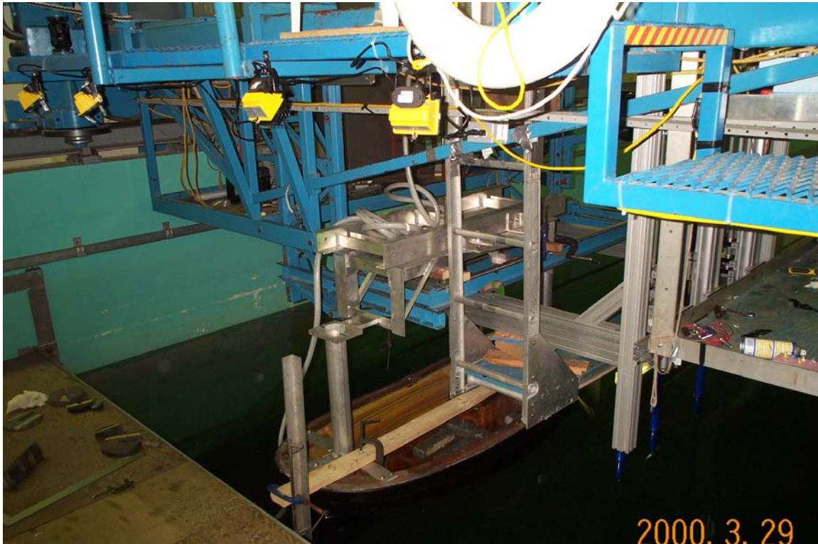
Figure 24, Model connected to OERC towing carriage, measurement plane at aft location
