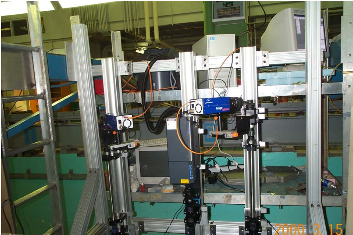
Figure 16, View of PIV system installed on OERC carriage.
