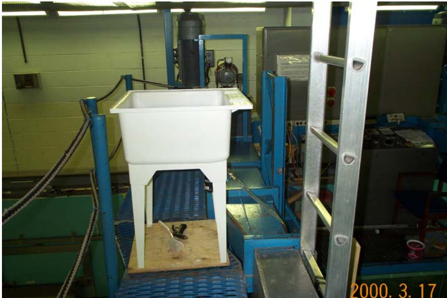
Figure 12, PIV seeding tank installed on OERC towing tank carriage
