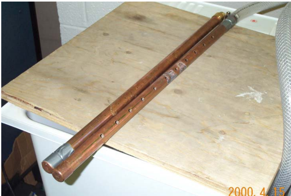
Figure 13, Seeding rakes (rake with large diameter holes on right)
