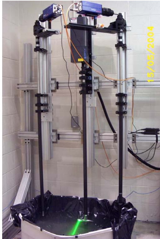
Figure 5, Small test tank and PIV equipment
