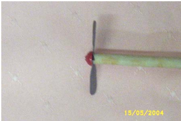
Figure 6, Small propeller model used for preliminary PIV experiments
