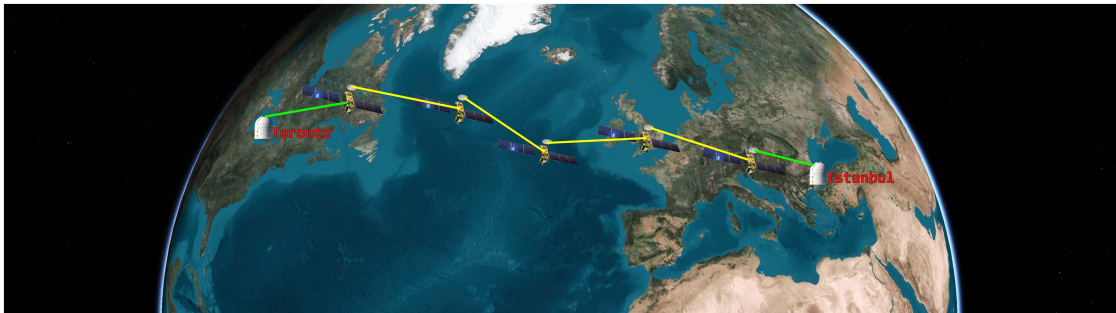
FIGURE 2. Illustration of a shortest path for a shorter LISL range for an inter-continental connection from Toronto to Istanbul.
