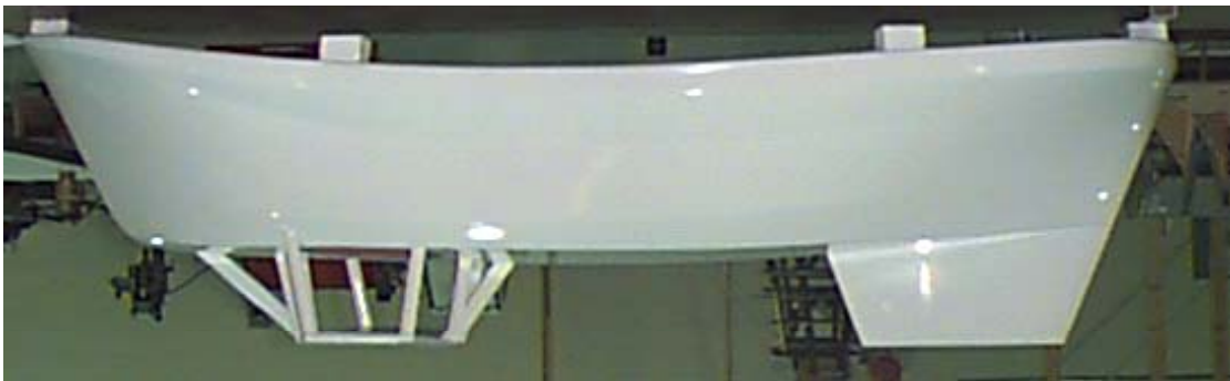
Figure 2, Side view of escort tug, showing low aspect ratio fin and propeller protection cage
