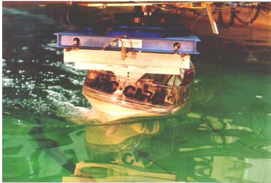
Figure 3, Model tested on PMM (10 knots)
