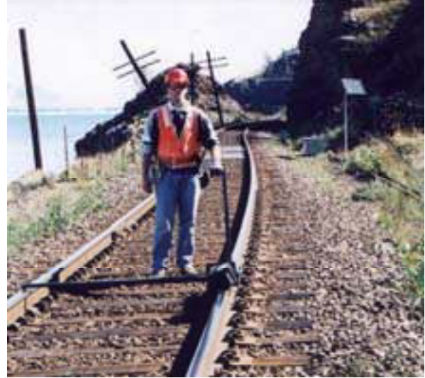
Figure 1: B) Hand operated tribometer used on CPR. The Portec solar-powered, electronic lubricator is shown in the background
