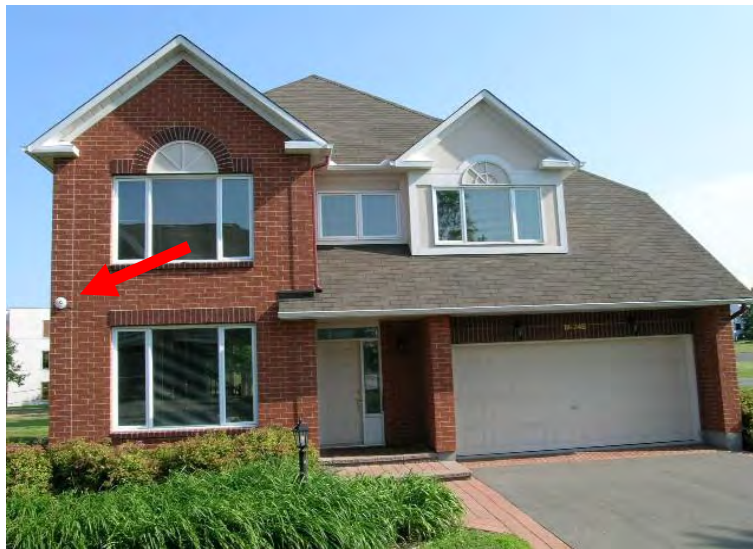
Figure 8 – South face of CCHT Reference House, showing location of the precision spectral pyranometer to measure incident solar radiation.
