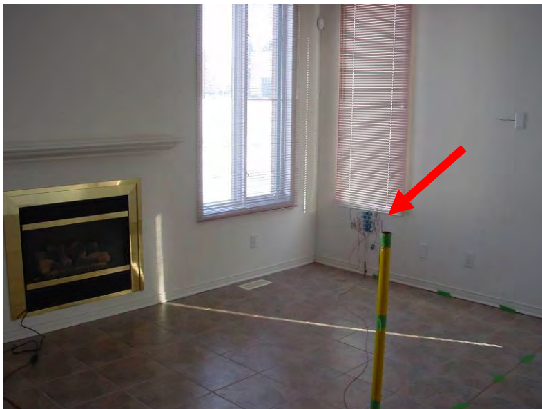
Figure 6 - Air temperature measurement in the family room
