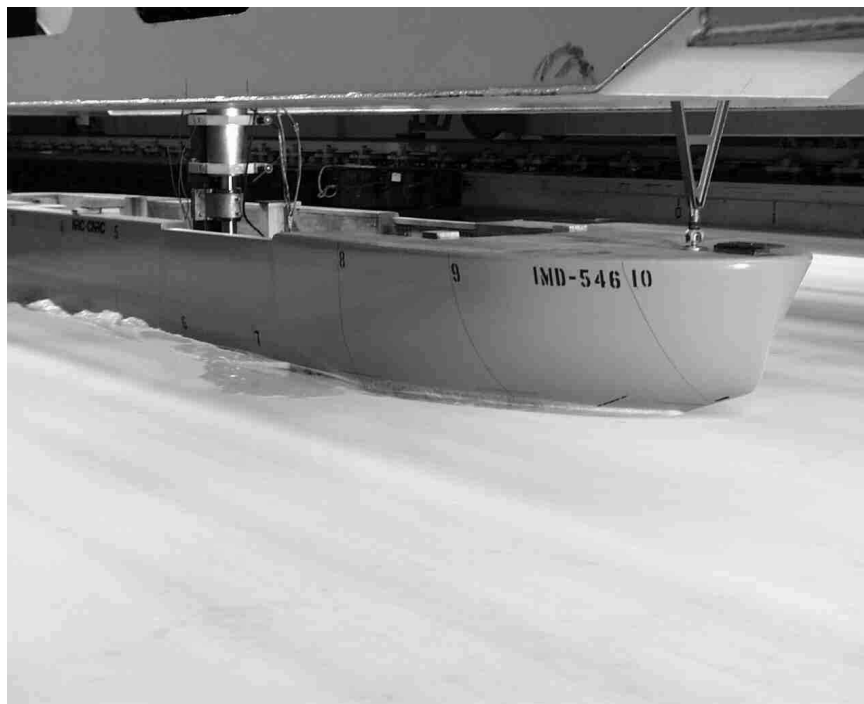
Figure 1: The USCGC Healy 1:23.7 scale model in the IMD ice tank.
