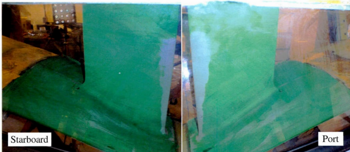
Figure 14: Paint removal on strut after 1 minute of spray with no IGVs installed
