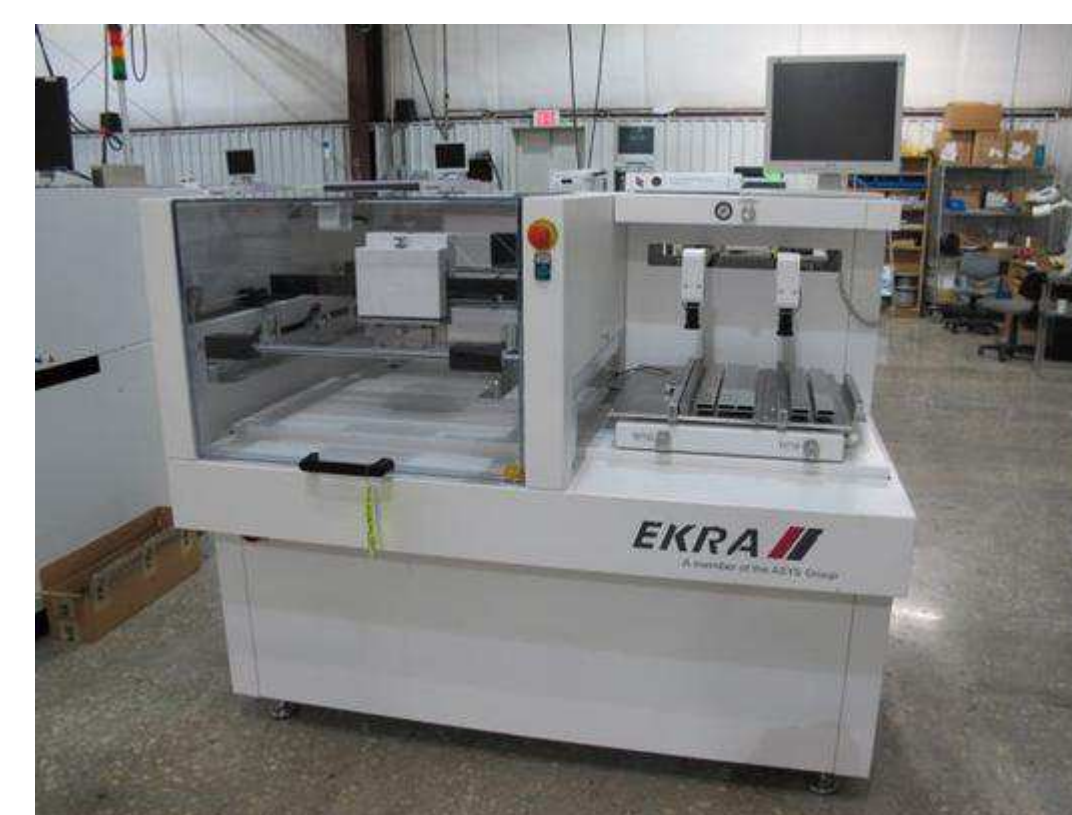
Fig. 2 Picture of the screen printer employed in this work
