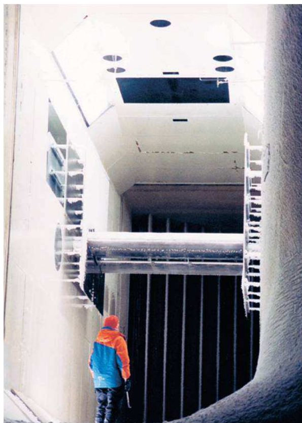
Figure 3.2: Snow simulation in the NRC 3 m × 6 m Propulsion and Icing Wind Tunnel
