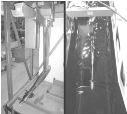
Figure 4. Kempf & Remmers dynamometer: in test frame (left) and in the tow tank (right).
