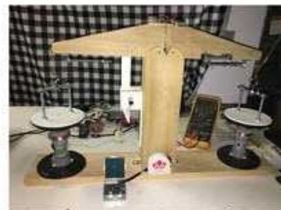
The McClure basement balance uses guidance on setup from the U.S. National Institute of Standards and Technology.
